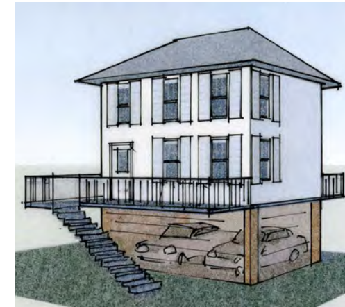
These proposed Terrytown housing designs illustrate the use of raised living areas utilized as parking to protect against flooding, and a hip-style roof which can resist high winds.
