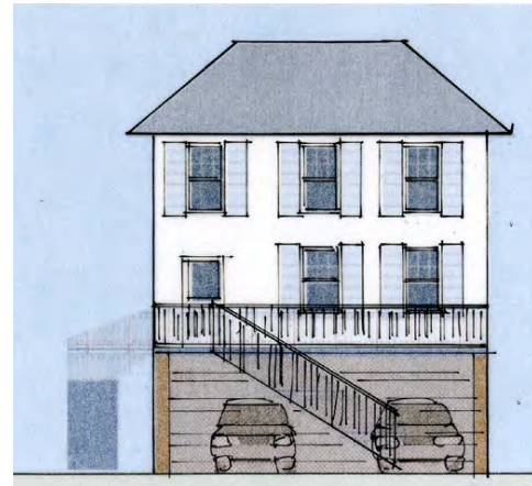
These proposed Terrytown housing designs illustrate the use of raised living areas utilized as parking to protect against flooding, and a hip-style roof which can resist high winds.
