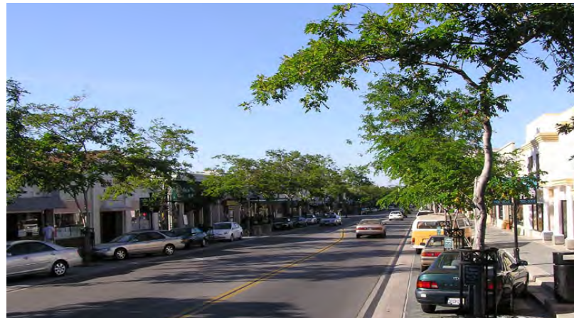
Stumpf Boulevard could look more like this pedestrian-friendly street in Mountain View, California, with street-level storefronts, on-street parking, trees, and a buffered sidewalk. 1
