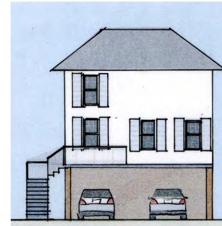
These proposed Terrytown housing designs illustrate the use of raised living areas utilized as parking to protect against flooding, and a hip-style roof which can resist high winds.
